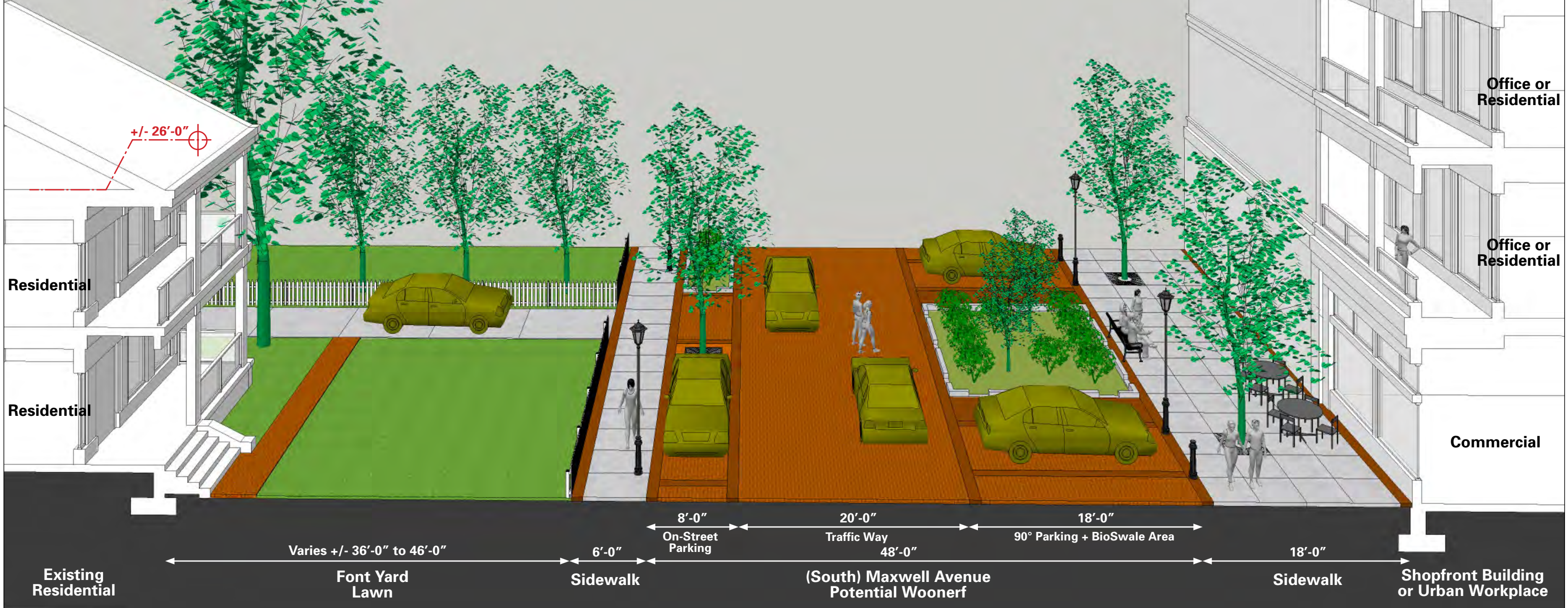
FIGURE 27: Conceptual Vision Plan: Southwest Quadrant - Conceptual Spatial Enclosure (Building Frontage/Form and Street Section) and Streetscape at S Maxwell Avenue (Segment B): Potential Woonerf (Living Street - Shared Space) Street Type.
