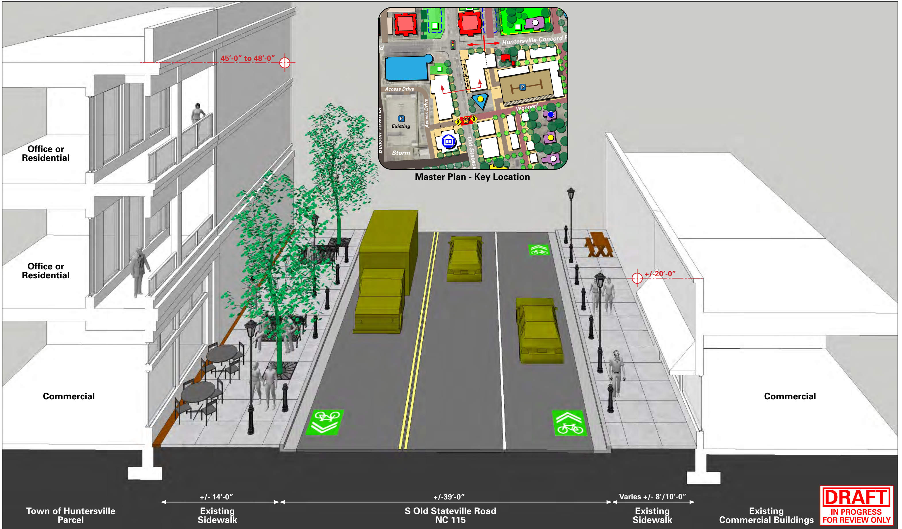
FIGURE 19: Conceptual Vision Plan: Southwest Quadrant - Conceptual Spatial Enclosure (Building Frontage/Form and Street Section) and Streetscape at S Old Statesville Rd: Potential Scenario A.
