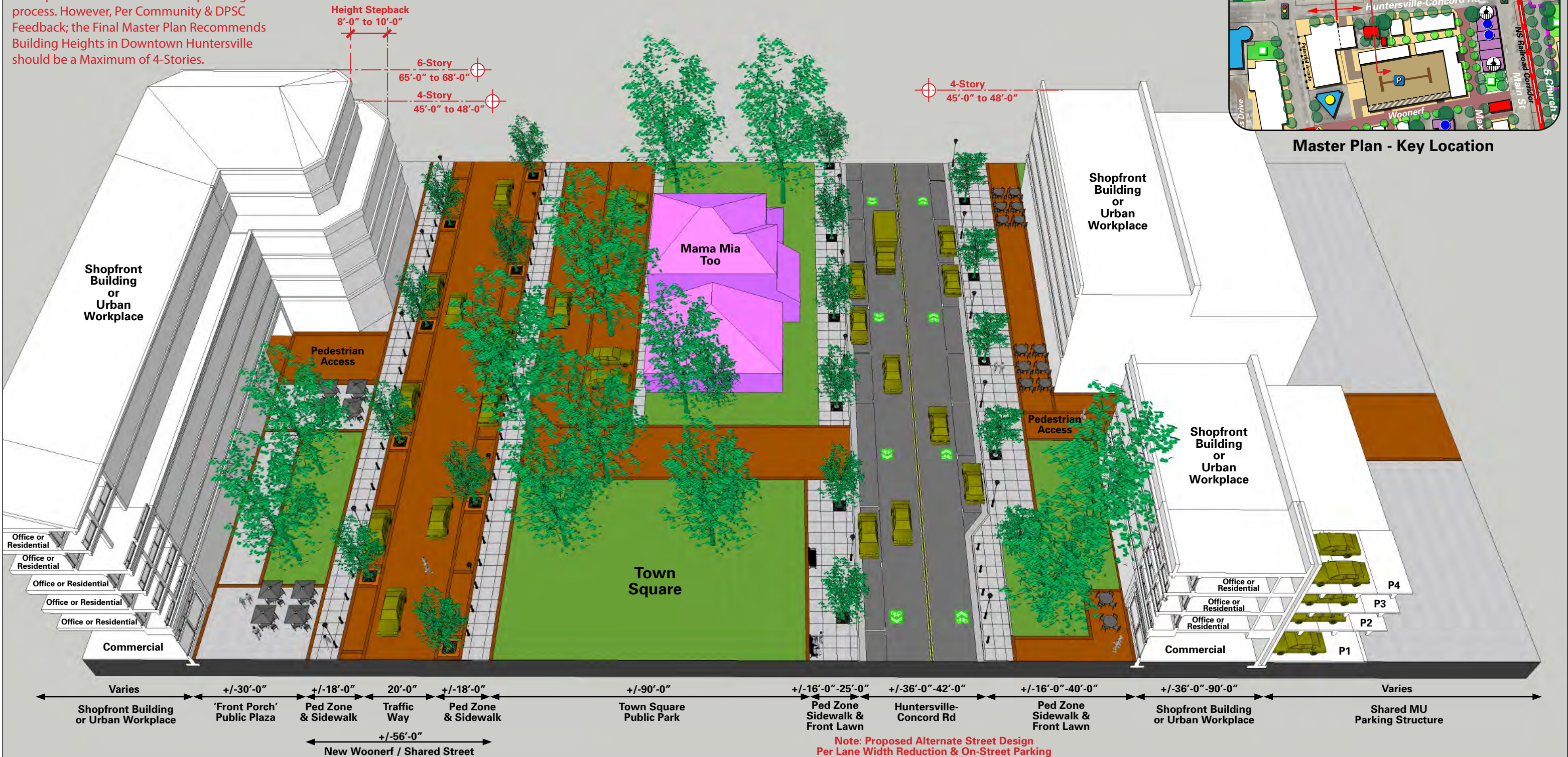
FIGURE 3: Conceptual Vision Plan: Northwest Quadrant - Conceptual Spatial Enclosure (Building Frontage/Form and Site/Street Section) and Streetscape at Proposed Town Square along Huntersville-Concord Road: Option A1.
