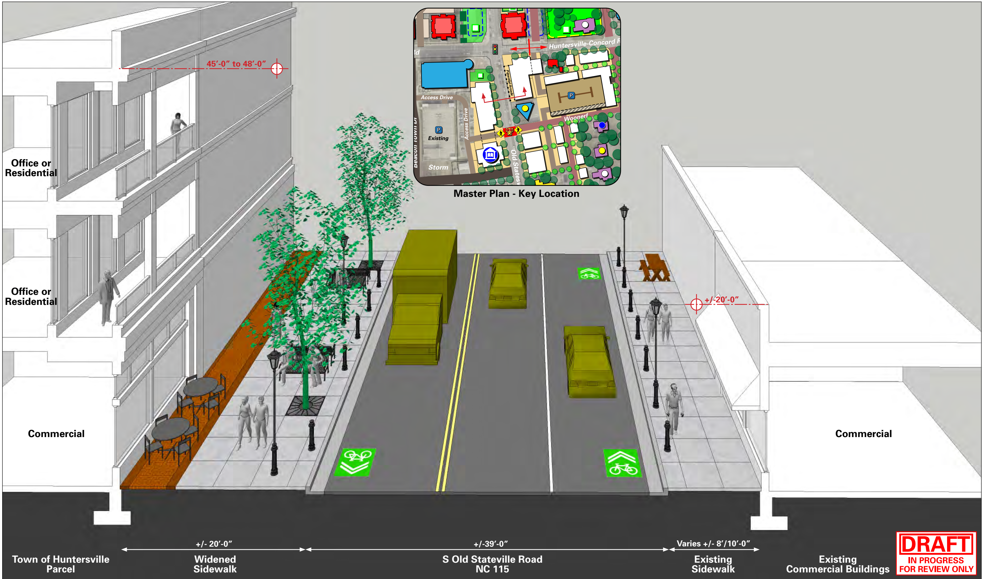
FIGURE 20: Conceptual Vision Plan: Southwest Quadrant - Conceptual Spatial Enclosure (Building Frontage/Form and Street Section) and Streetscape at S Old Statesville Rd: Potential Scenario B.
