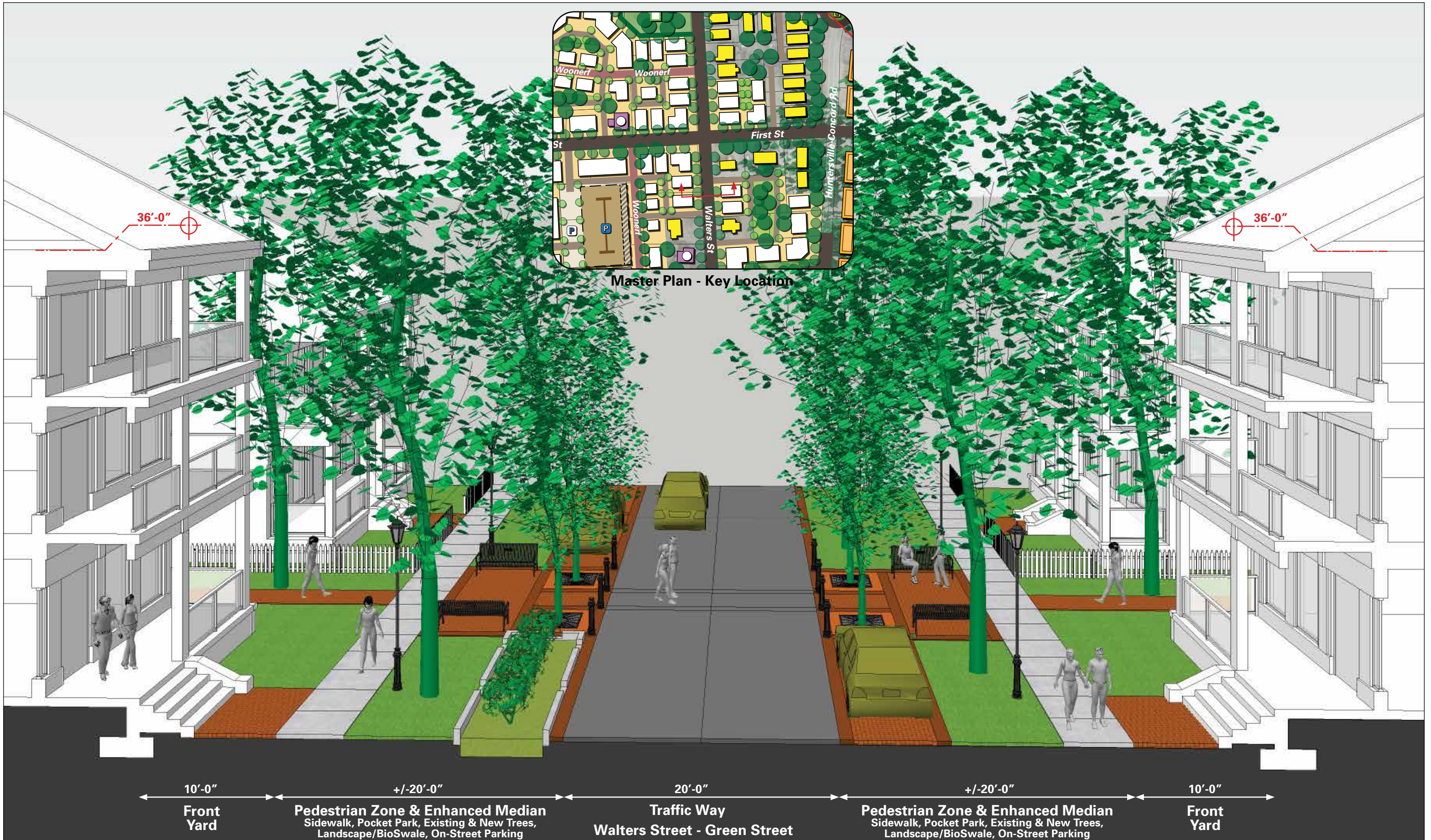
FIGURE 16: Conceptual Vision Plan: Northeast Quadrant - Conceptual Spatial Enclosure (Building Frontage/Form and Site/Street Section) and Streetscape at Walters Street - Proposed 'Green Street' Improvements: Apartment (Tri/Quad) Building/Lot Types.
